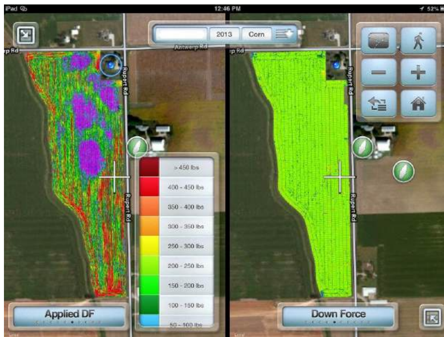
Fig. 11. Delta Force system with FieldView option
