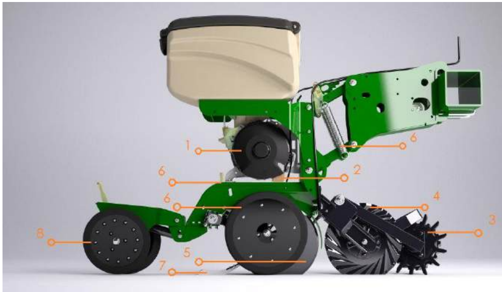
Fig. 1. Section of the seeder of precision seeding: 1 – construction of the seeding device, 2 – vas deferens, 3 – unfolds, 4 – turbodisc, 5 – opener, 6 – sowing depth adjustment system, 7 – seed sealer, 8 – rolling wheels
